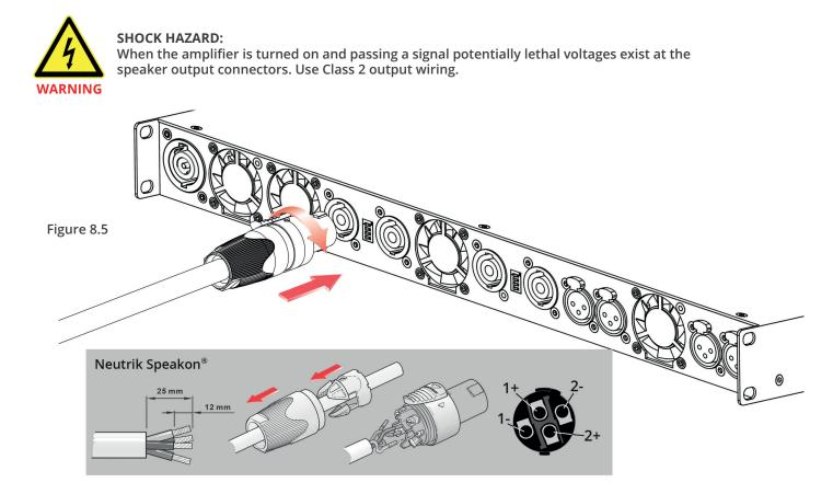
Select the appropriate size of wire based on the distance from amplifier to speaker.
