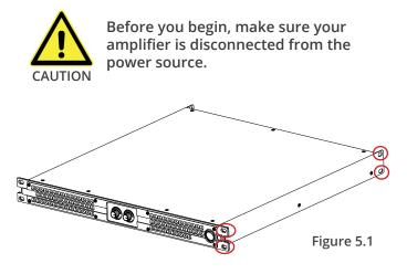
The common installation of the SX-Amplifier Series is in 19" standard rack cabinets. In order to limit the risk of mechanical damages, the amplifiers must be fixed to the rack using both frontal and rear mounting brackets. (See Figure 5.1)
