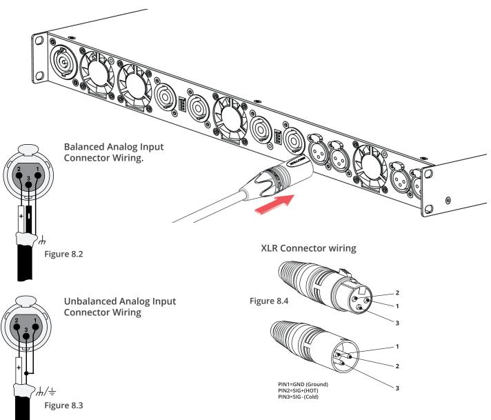
The cable quality has a major impact on the sound quality of your entire audio system. Take care to always use high quality shielded wire cable for input wiring. The higher the density of the shield the better. Spiral wrapped shield should be not used.
